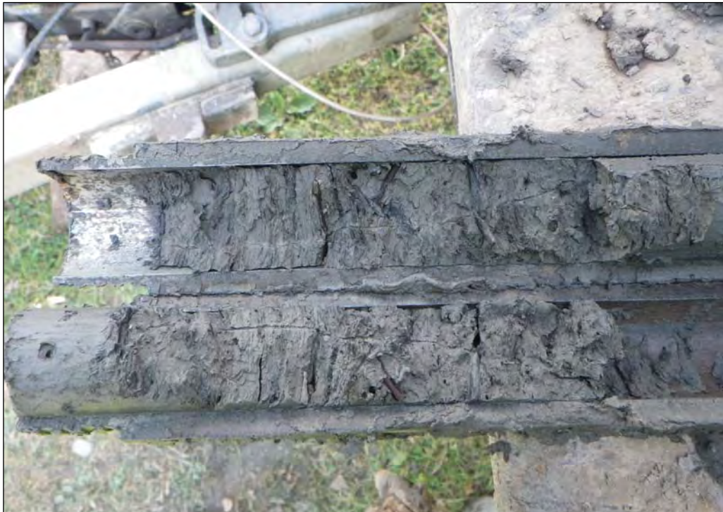
Plate 46: Alluvial deposits within BH04 at 8.5m to 8.95m BGL
