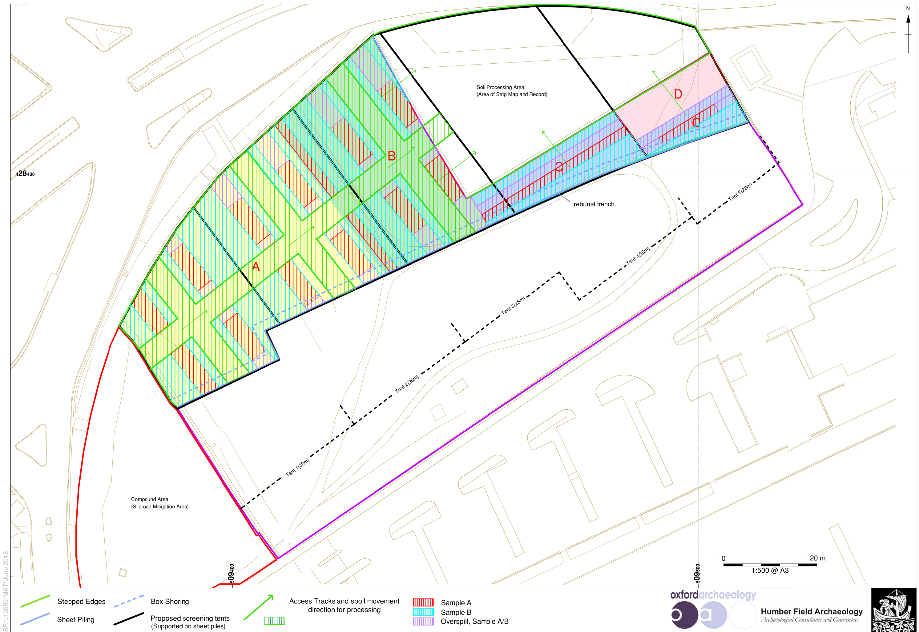
Figure 4: Plan showing proposed access tracks, piling and sampling areas for the recovery of 1500 skeletons for analysis
